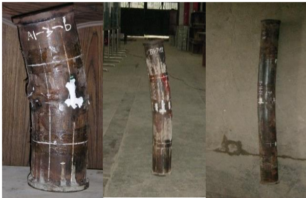
Figure 2: Typical failure modes of specimens
